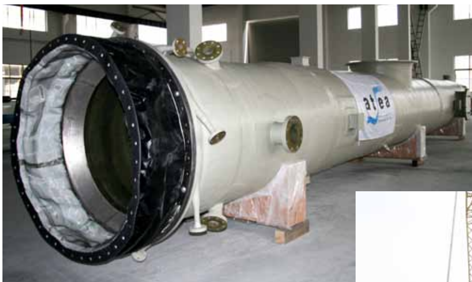
Quench Tower Diameter: 1,200mm Height: 11,300mm
