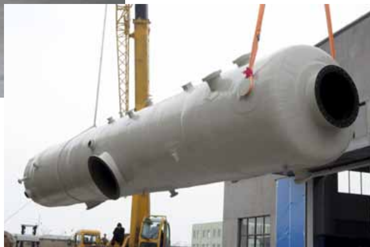
Scrubber Diameter: 2,000mm Height: 11,700mm
